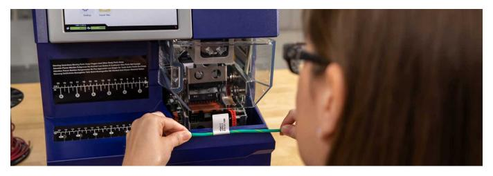
Experienced operators can print and manually apply a flag label on a cable in 15 seconds. With the BradyPrinter A5500 Flag Printer Applicator they can significantly increase production output by flagging cables in 5 seconds.
