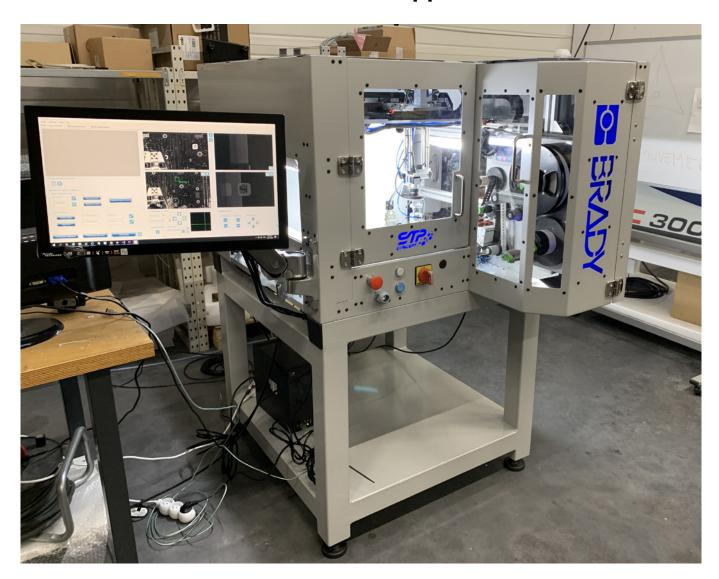
Automatically print & place a reliable traceability label anywhere on any multi- or single board standard PCB in 3 seconds.
