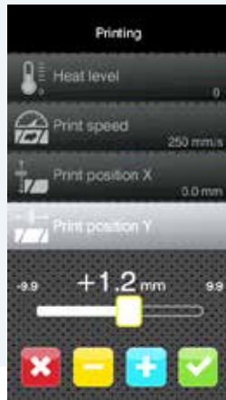
Print position Y Fast setup with a slider, fine setup with ± keys
